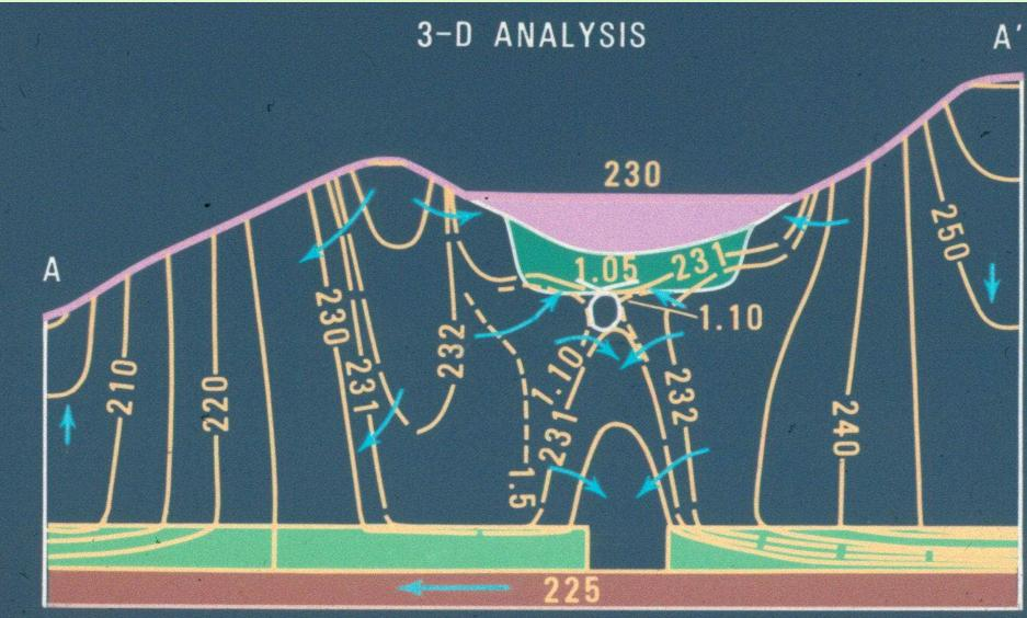
What if the rubble in the hole is really dirty (lower-*K*)? Now the lake stops losing water and a closed flow system develops.
