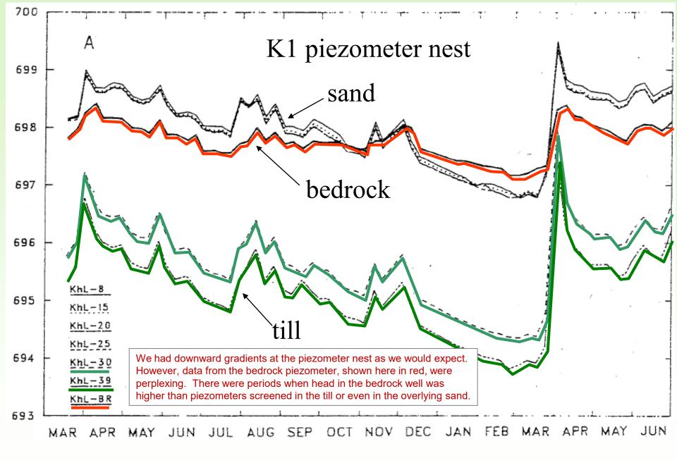
High bedrock head suggests upward GW flow at downgradient side of lake <sup>15</sup>
