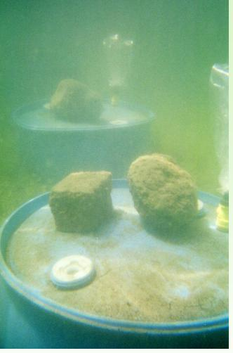
Seepage limited by a 20-30 cm thick clogging layer of sand with some organics Rosenberry, 2000, *WRR*  Measured seepage ranged from 0.1 to 263 and averaged 37 cm/d
