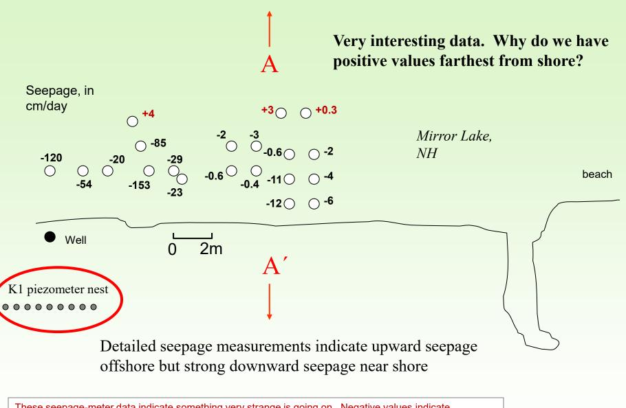
These seepage-meter data indicate something very strange is going on. Negative values indicate downward seepage and positive values indicate upward seepage. The meters farthest from shore indicate upward seepage but everything else closer to the shoreline indicates downward seepage, including some very fast rates of downward seepage. Interesting. What do data from the piezometer nest show?
