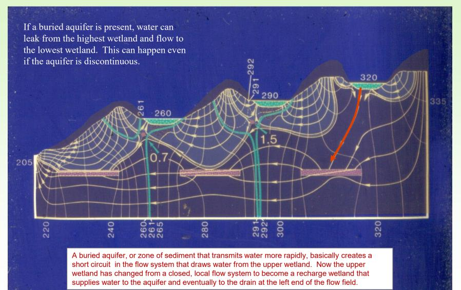
A stagnation point (blue dot) forms at the point where head along a flow-separation line is lowest. A stagnation point is a point in a flow field of zero velocity. Ground water is not moving at a stagnation point. (Water could be very old near a stagnation point and interesting chemistry could result.)
