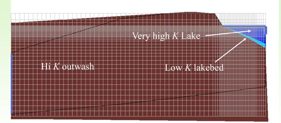
The organic-rich sand of the lakebed was simulated in the light blue zone that increased in thickness with distance from shore. This is under the assumption that waves at the shoreline would wash fine-grained particles into the lower-energy deeper portions of the lake.
