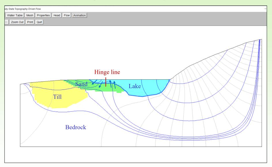
Notice the flow line that enters the lake, flows laterally through the lake, and then leaves the lake to flow downward into the sand. That key flowline is proof that a hinge line exists that separates upward flow of groundwater to the lake from downward flow from the lake to groundwater.
