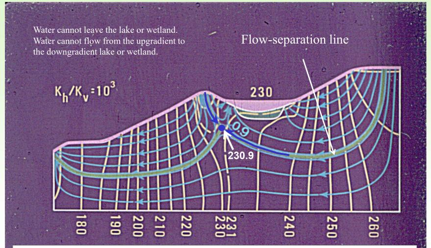
If a stagnation point is present, a closed, local flow system exists. Water cannot leave the wetland; water cannot flow from the wetland to a lower-head drain. Tom Winter was very excited to discover the concept of stagnation points, but it turns out petroleum engineers had known about this years earlier. But no one had thought about this from a groundwater-surface-water perspective. Luckily, Tom's advisor was well versed in the petroleum-engineering literature.
